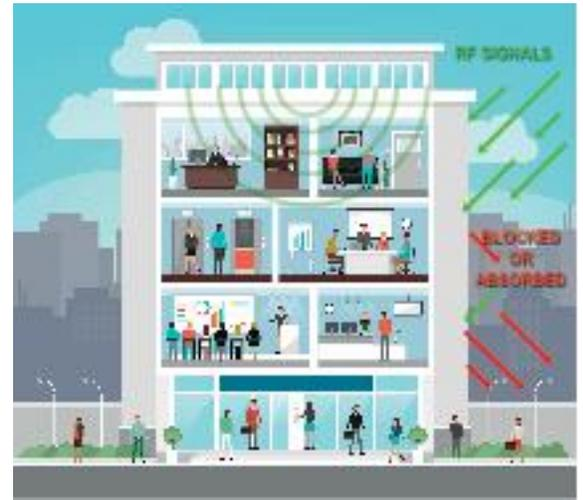
**An In-Building Public Safety Communication System** enhances radio signals so they are available throughout the building, including areas that are especially difficult for RF to penetrate such as stairwells, elevators, basements, and thick-walled or shielded areas.
